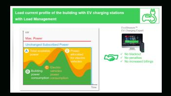
"This system is designed to optimize the distribution and consumption of electrical power among multiple EV chargers. It dynamically adjusts the power allocated to each charger based on real-time demand and pre-set priorities, ensuring efficient energy use without overloading the electrical network "
